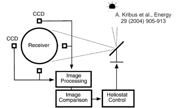
The heliostat control loop is closed by acquisition of four images around the receiver aperture, and generating a control signal by image processing.
